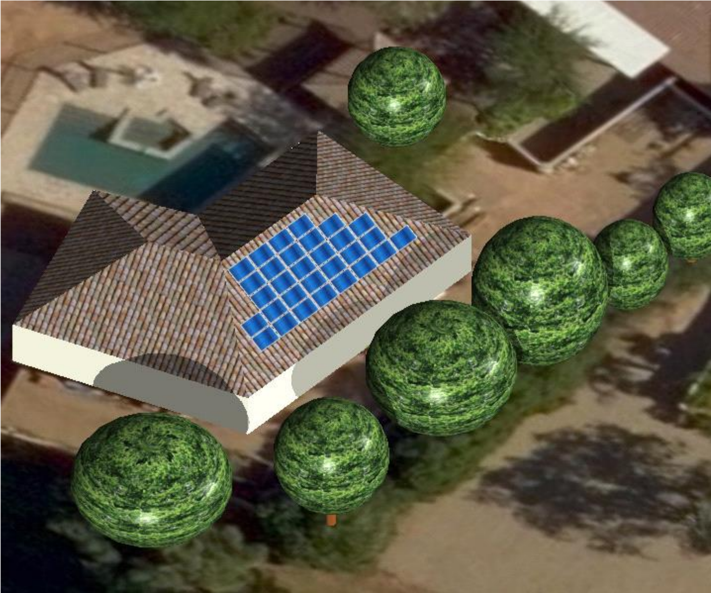
Figure 3: Realistic view of system installation
